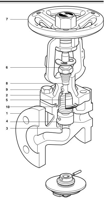
Optional balancing disc assembly 10 bar ∆P DN200 Used above
